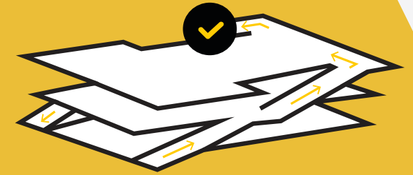
Flat Floors (one way ramps): Structures with flat floors and one-way ramps minimize sloped floor space to maximize future re-use.
